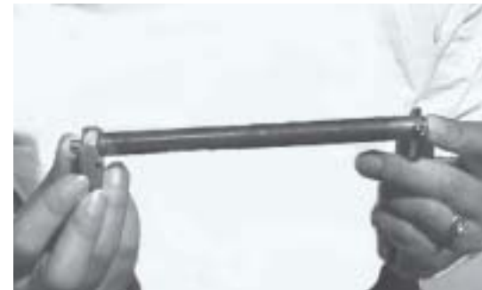
Adjusting the Length of a Quick Release Axle
