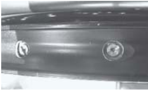
Double-wall Rim with Recessed Spokes and Nipples
